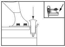
Figure 1. Releasing magazine latch.
